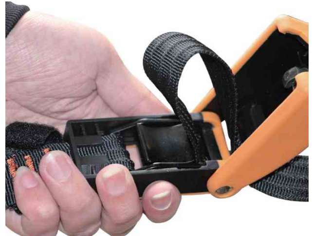
STEP 4 AND THEN THE EXTRA STRAP STRETCHES OUT FROM THE LID.
